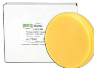
Extremely stable milling wax discs made from temperature stabilised micro wax. Burns out without leaving residue, milled parts have mirror-smooth even surfaces. Dropping point of 120°C - wax chippings can be easily vacuumed off without melting.
